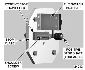
**Kettle Fully Tilted - Traveller Contacts Stop Plate**
